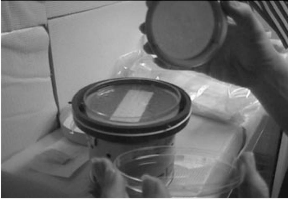
*Figure 4.3-2 Burkard air sampler being prepared for sample collection*
