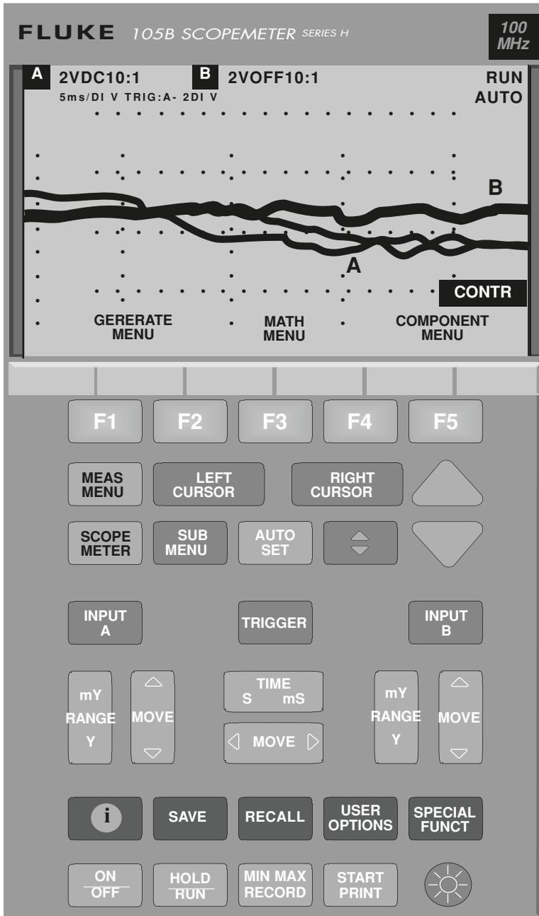
*Figure 6.2-3 The Fluke ScopeMeter, an electrical diagnostic instrument*
