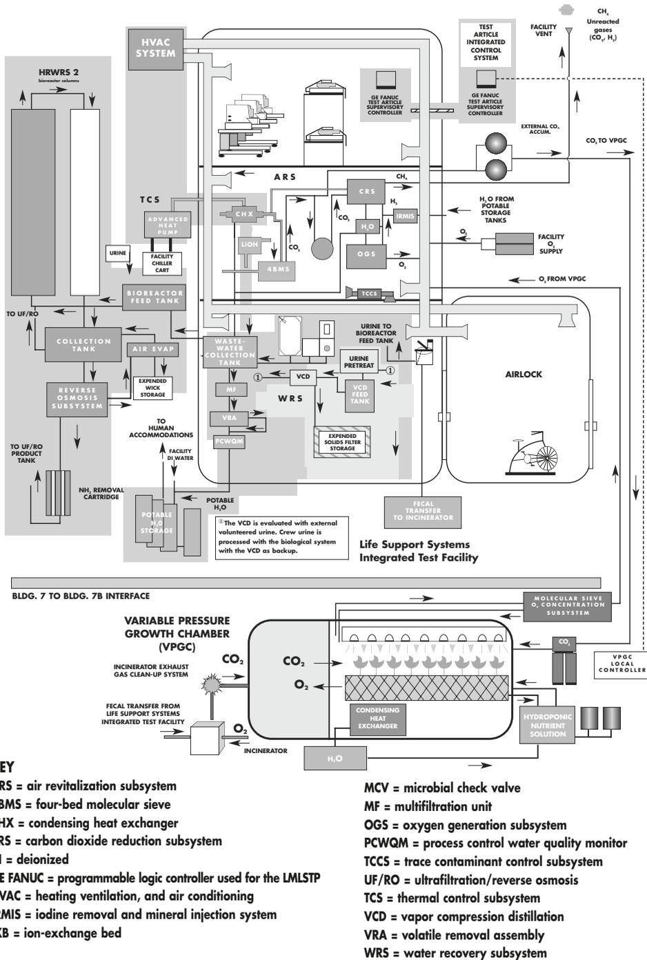
Figure 2.1-6 The Phase III, 91-day test functional schematic
