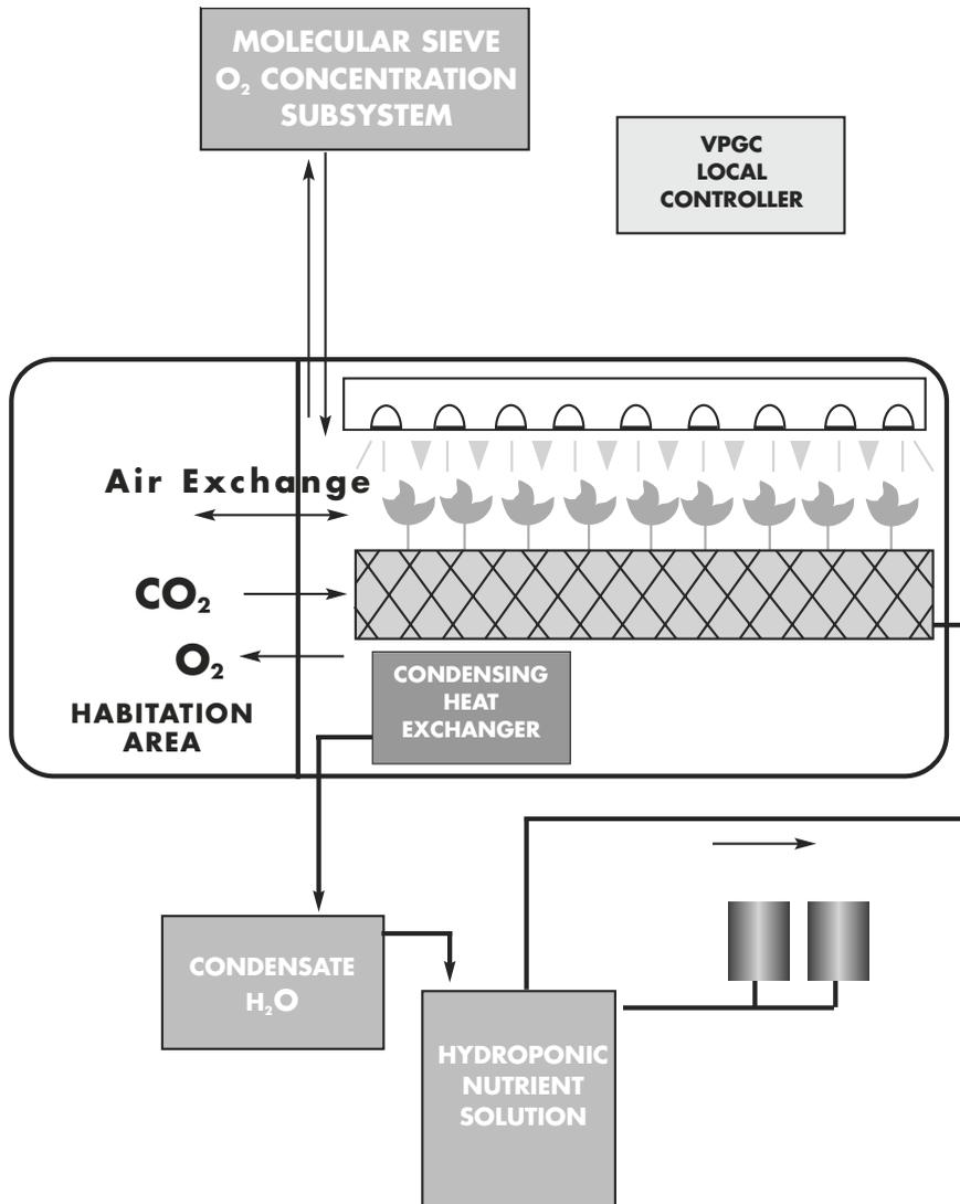
*Figure 2.1-2 The Phase I, 15-day test functional schematic*
