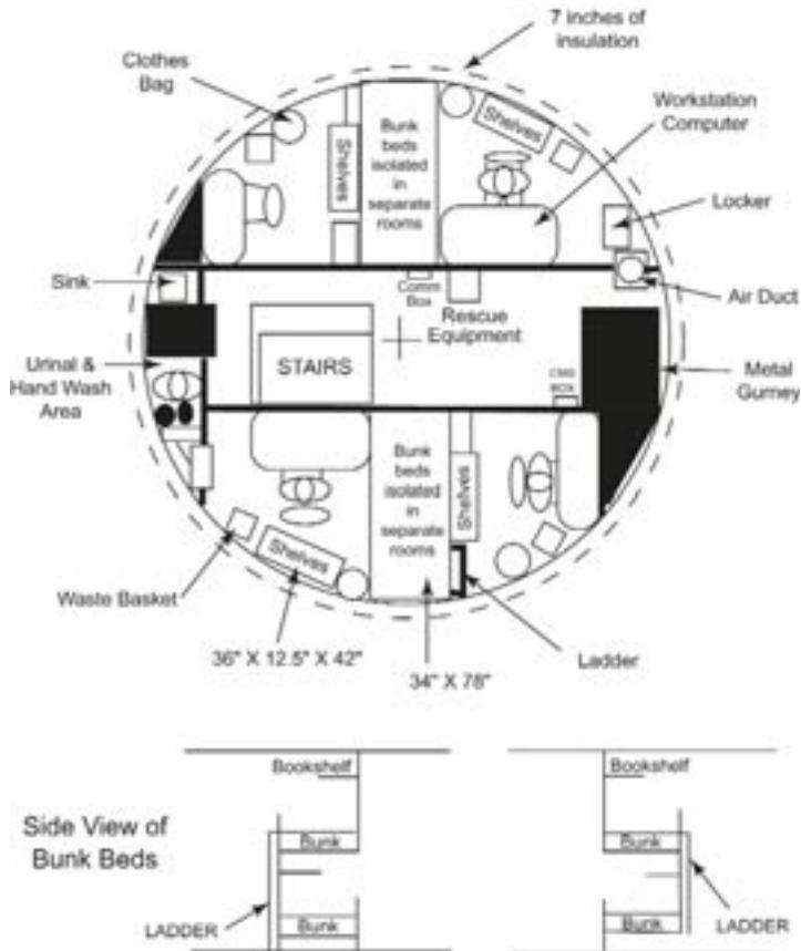
**Figure 3.1-18** Floor plan for third level of chamber. Detail of bunk area illustrates the utilization of the bed from each crew quarter
