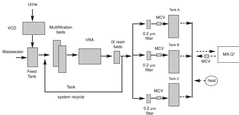
*Figure 4.2-2 Phase IIa Recovery System Schematic*
