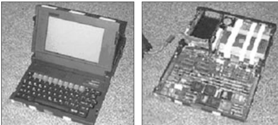
*Figure 6.2-2 The GRiD computer. The left photo shows the assembled computer. The right shows a stage midway through the assembly*
