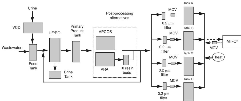
*Figure 4.2-1 Phase II Water Recovery System Schematic*
