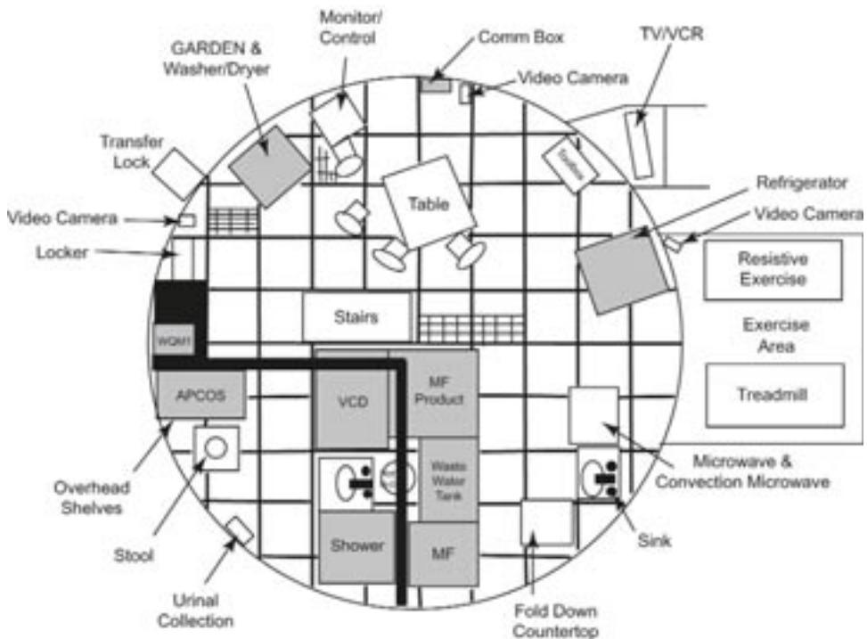
*Figure 3.1-6 LLSIF lower level floor plan*
