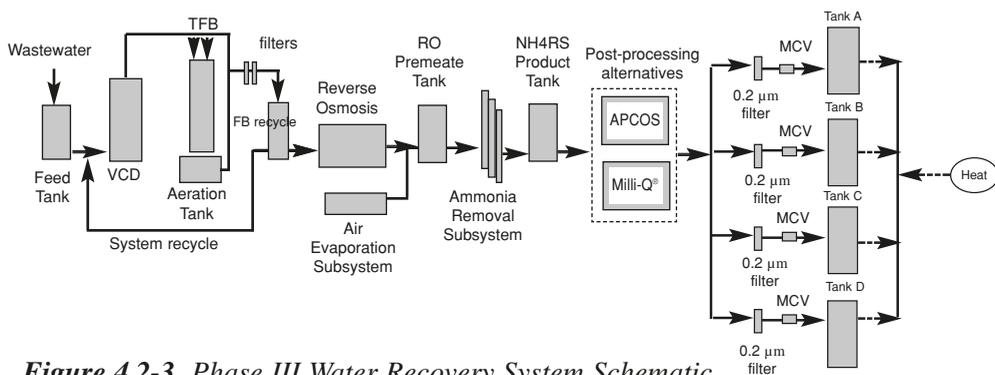
**Figure 4.2-3** Phase III Water Recovery System Schematic
